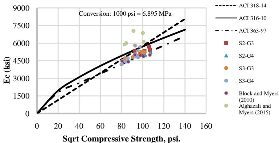
Figure3. Modulus of elasticity vs. compressive strength
