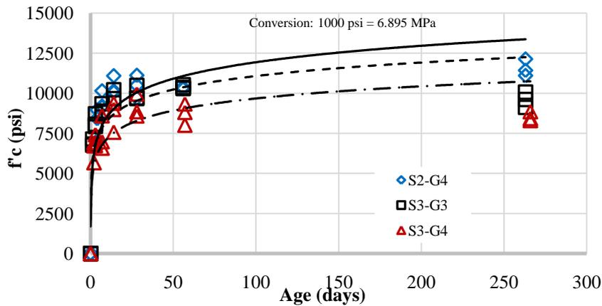
Figure 2. HS-SCC Compressive Strength Results
